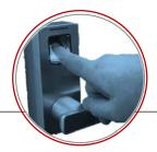
**Bio-entry Readers** – Fingerprint readers from Suprema are able to be integrated with Millennium Ultra, allowing for a card-less access. The cardholders can be assigned fingerprints all from within Ultra.
